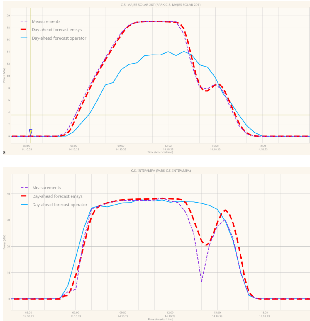
FIGURE 20. Plant operators not incorporating the solar eclipse in their production forecast
